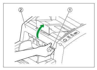
3. Push in both sides of the paper feed roller cover, and pull it towards you to open.
